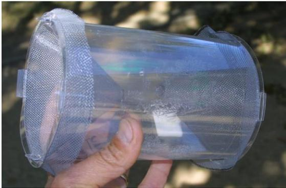
Figure 2. Improved version of the experimental Trece double cone trap, with a plastic ring fitted to top and bottom to secure the cone screen on top and bottom instead of a rubber band and staples. This trap has adhesive on the inside to keep BMSB in the trap.
