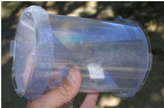
Figure 3. Improved version of the experimental Trece double cone trap, with a plastic ring fitted to top and bottom to secure the cone screen on top and bottom instead of a rubber band and staples. This trap has adhesive on the inside to keep BMSB in the trap.
