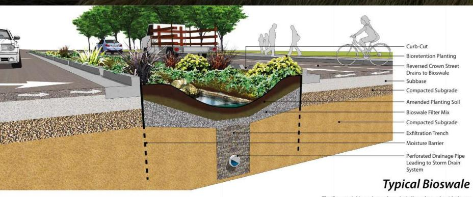
The Cannery's bioswales are broad, shallow channels with dense vegetation covering the side slopes which provides filtration and reduces flow velocities as the runoff is conveyed through the system. These swales function as part of the stormwater conveyance system and can potentially reduce the need for curbs, gutters and storm drains.
